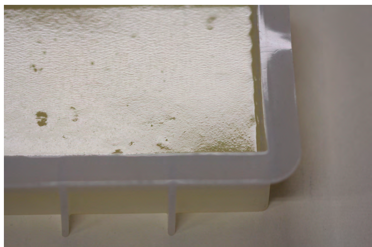
Fig. 1: Silicone tray, 10x15x5 cm, to prepare the gels and thickener. Silicone provides a smooth and non-adhesive surface.
