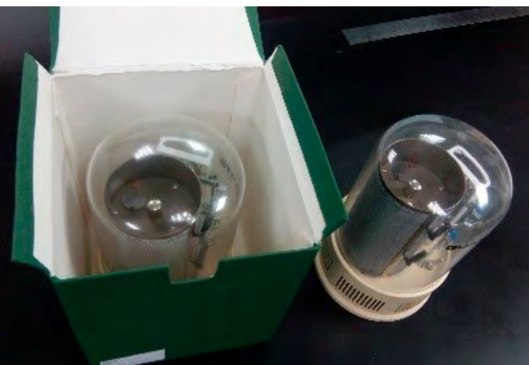
Fig. 2: Two Quartz Domed mini drum hygrothermographs, one inside a Buckram-cloth covered box and another outside.
