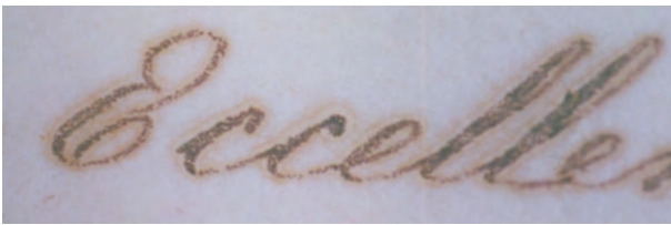
Fig. 4: Schliemann's archive, the Gennadius Library. Volume BBB27, page 415, visible photography (VIS), close-up. Each character is surrounded by a diffusion halo and a boundary halo around the diffusion one.
