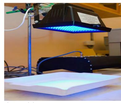
**Fig. 1:** Spotlight SP–S 180-20-220 with 180 blue LEDs
