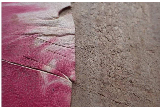
Fig. 7: XI 628 red alum tawed sheep skin, irregular turn-in cut, edge of dyeing, scratches and cuts on leather and wood, wood beach, direction parallel to spine.
